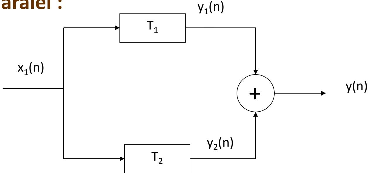
$$y(n) = y_1(n) + y_2(n) = T_1[x(n)] + T_2[x(n)]$$
